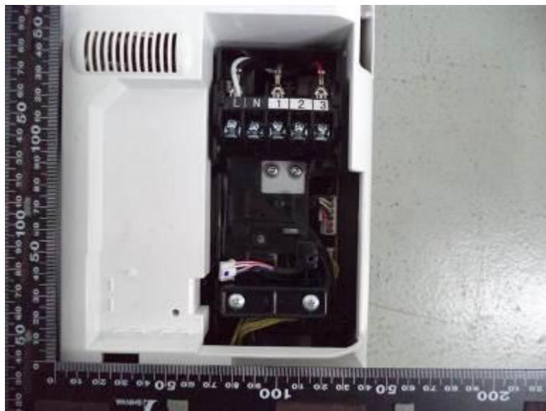
75. RAS-B22PKVSG-E,RAS-B22PKVSG-TR,RAS-B24PKVSG-E,RAS-B24PKVSG-TR, Terminal supply, interconnecting terminal and cord anchorage
